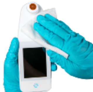
Figure 28 Clean the Front of the Scanner
