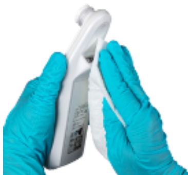
Figure 26a Clean the Sides and Back of the Scanner
