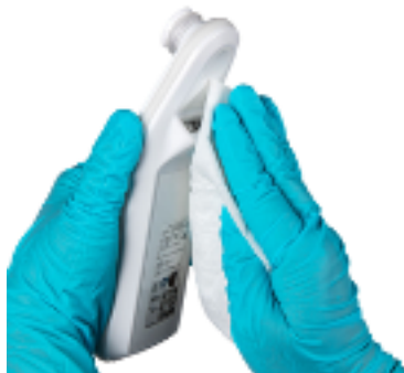
Figure 27 Clean the Sides and Back of the Scanner
