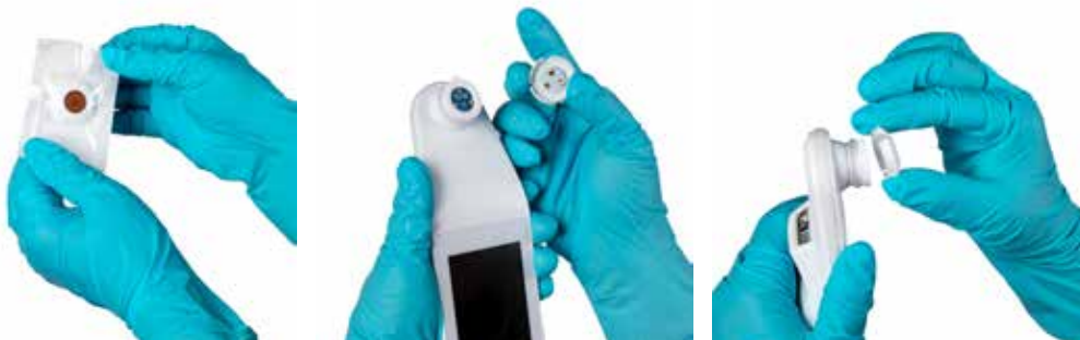
Figure 14 Installation of the Single-Use Sensor
