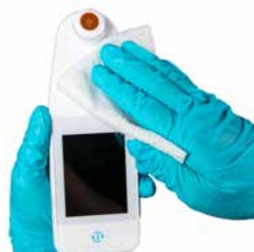
Figure 27 Disinfect the Front of the Scanner
