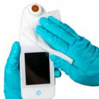
Figure 25 Clean the Front of the Scanner
