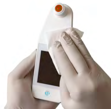
Figure 26. Disinfect the Front and back of the SEM Scanner
