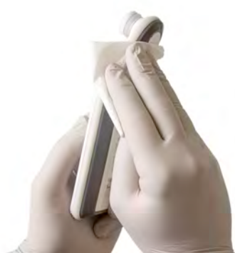
Figure 25. Disinfect the Sides of the SEM Scanner
