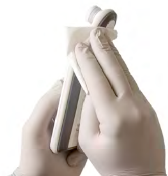
Figure 23. Clean the Sides of the SEM Scanner
