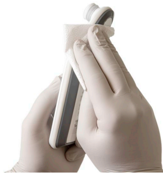
Figure 23. Clean the Sides of the SEM Scanner
