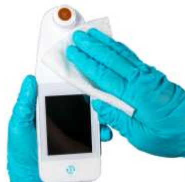
Figure 27 Disinfect the Front of the Scanner
