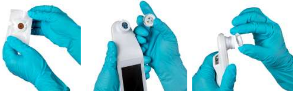
Figure 14 Installation of the Single-Use Sensor
