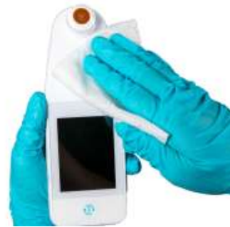
Figure 25 Clean the Front of the Scanner
