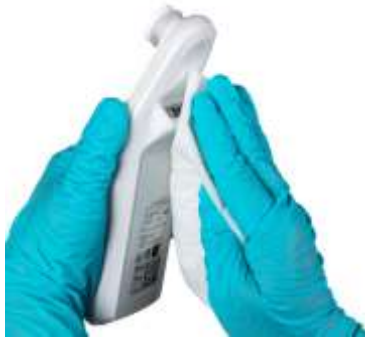
Figure 24 Clean the Sides and Back of the Scanner
