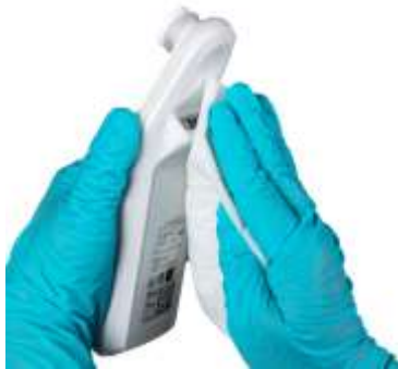
Figure 26 Disinfect the Sides and Back of the Scanner
