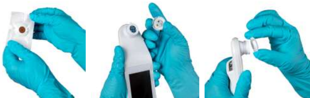
Figure 14 Installation of the Single-Use Sensor
