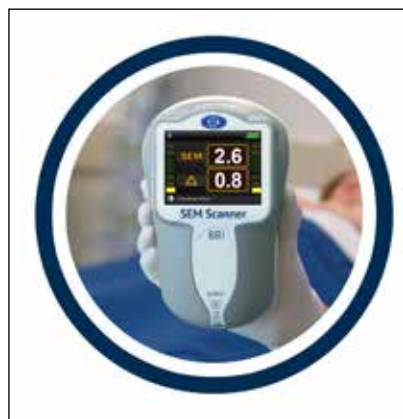
Figure 2. SEM scanner display showing the delta ( \Delta ) value
