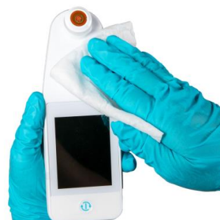
Figure 25 Clean the Front of the Scanner
