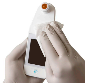
Figure 24. Clean the Front and back of the SEM Scanner
