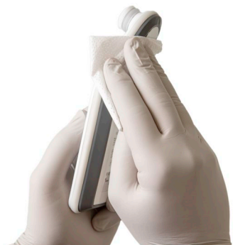
Figure 23. Clean the Sides of the SEM Scanner
