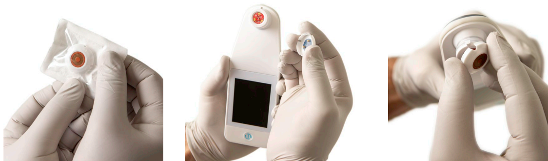
Figure 14 Installation of the Single-Use Sensor
