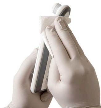
Figure 25. Disinfect the Sides of the SEM Scanner
