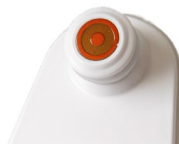
Figure 9 Sensor of the Provizio SEM Scanner
